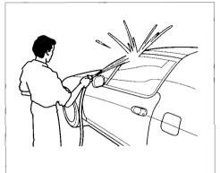
A high pressure water stream can distort the roof seals and cause them to leak. Do not spray a high pressure stream from a hose directly at the roof seals.
