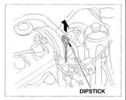
Check the engine oil level every time you fill the car with fuel. Wait at least two minutes after turning the engine off before you check the oil.
