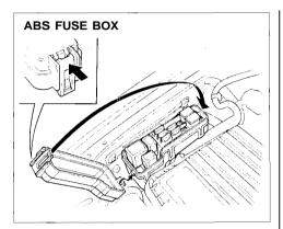
Cars equipped with ABS have a third fuse box for the ABS. It is in the front of the engine compartment on the passenger's side.
