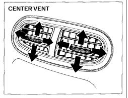
You can adjust the direction of the air coming from the dashboard vents by moving the tab in the center of each vent up-and-down and side-to-side.
