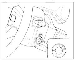
The ignition switch is on the right side of the steering column. It has four positions: LOCK (0), ACCES-SORY (I), ON(II), and START (III).
