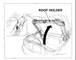
You cannot put any luggage in the trunk without lifting up the roof holder when the roof is stored in the trunk.
