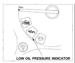
This indicator should light when the ignition is ON (II), and go out after the engine starts. It should never come on when the engine is running. If it starts flashing, it indicates that the oil pressure dropped very low for a moment, then recovered. If the indicator stays on with the engine running, it shows that the engine has lost oil pressure and serious engine damage is possible. In either case, you should take immediate action.
