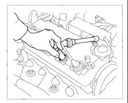
5. Put the new spark plug into the socket, then thread it into the hole. Screw it in by hand so you do not crossthread it.
