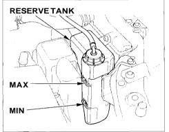
Check the level of the engine coolant by looking at the radiator reserve tank near the right headlight. If the coolant level in the reserve tank is at or below the MIN line, add coolant to bring it up to the MAX line. Inspect the cooling system for leaks. This coolant should always be a mixture of 50% antifreeze and 50% water. Never add straight antifreeze or plain water.
