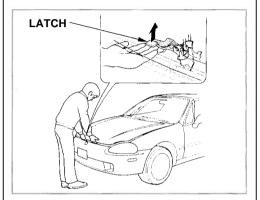
2. Standing in front of the car, put your fingers under the front edge of the hood to the left of center. Slide your hand to the right until you feel the hood latch handle. Push this handle to the right until it releases the hood. Lift the hood.
