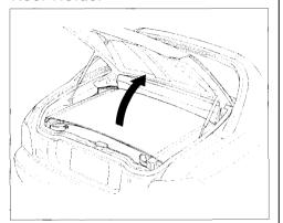
To reach items in the trunk when the roof is stored, pull the roof holder lock lever and lift the holder.
