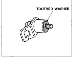
The anchor plate and mounting hardware for a top tether are supplied with the car. When installing, make sure the toothed washer is on the bottom of the bolt.
