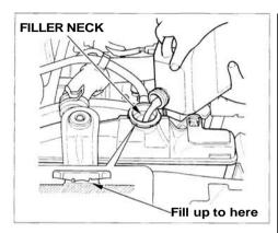
9. Pour coolant into the radiator up to the base of the filler neck.
