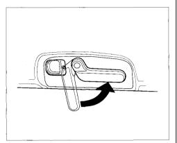
8. Secure the roof by turning each release lever until the lock tab clicks forward. Pull on the levers to make sure they are locked.
