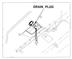
3. Loosen the drain plug on the bottom of the radiator. The coolant will come out through the hole in the splash cover.
