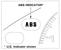
The ABS is self-checking. If anything goes wrong, the ABS indicator on the instrument panel comes on (see page 34). This means the Anti-lock function of the braking system has shut down. The brakes still work like a conventional system, providing normal stopping ability. You should have the dealer inspect your car as soon as possible.
