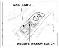
To open the passenger's window or rear window from the master control panel, push down on the appropriate switch and hold it down until the window reaches the desired position. To close the window, push up on the window switch. Release the switch when the window gets to the position you want.
