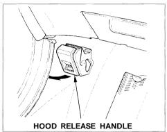
Shift to Park or Neutral and set the parking brake. Pull the hood release handle, located under the left lower corner of the dashboard. The hood will pop up slightly.
