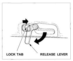
4. Release each side of the roof by pushing the lock tab sideways and pulling down the release lever. Carefully lift the roof straight up.
