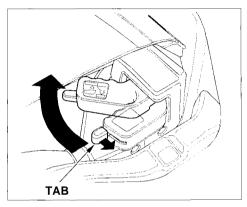
4. Release the roof from the holder by pushing the tabs and pivoting the lock levers forward.
