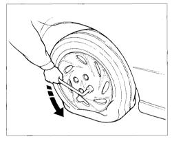
7. Loosen the four wheel nuts 1/2 turn with the wheel wrench.
