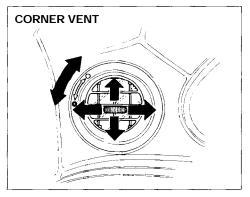
The corner vents and the center console vent on the driver's side can be closed by turning the vent approximately 45° clockwise.
