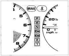
This display is on the instrument panel. It shows you the position of the shift lever.
