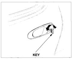
The doors can also be locked and unlocked from the outside with the key.
