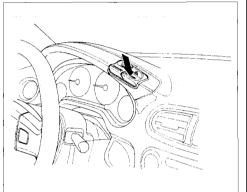
Push the red button on the dash above the instrument panel to turn on the hazard warning lights (fourway flashers). This causes all four outside turn signals and both indicators in the instrument panel to flash. Use the hazard warning lights if you need to park in a dangerous area near heavy traffic, or if your car is disabled.
