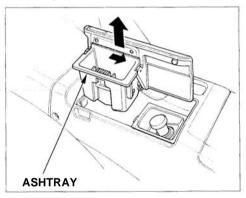
Open the ashtray by lifting the lid up. To remove it for emptying, open the lid then pull it straight out of the holder. To reinstall the ashtray, put it back in the holder with the lid open and push it straight down.
