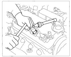
6. Torque the spark plug. (If you do not have a torque wrench, tighten the spark plug 2/3 turn after it contacts the cylinder head.) Tightening torque: 18 N.m(1.8kgf.m,13 lbf.ft)
