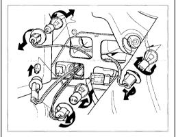
Determine which of the four bulbs is burned out: tail/stoplight, backup light, turn signal, or side marker. Remove the socket for that bulb by turning it counterclockwise.
