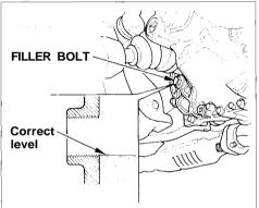
Check the fluid level with the transmission at normal operating temperature and the vehicle sitting on level ground. Remove the transmission filler bolt and carefully feel inside the bolt hole with your finger. The fluid level should be up to the edge of the bolt hole. If it is not, add genuine Honda Manual Transmission Fluid until it starts to run out of the hole. Reinstall the filler bolt and tighten it securely.
