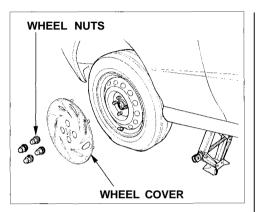
On Smodel Do not attempt to forcibly pry the wheel cover off with a screwdriver or other tool. The wheel cover cannot be removed without first removing the wheel nuts.
