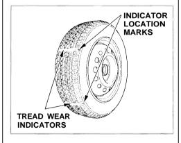
Your car's tires have wear indicators molded into the tread. When the tread wears down to that point, you will see a 12.7 mm (1/2 inch) wide band running across the tread. This shows there is less than 1.6 mm (1/16 inch) of tread left on the tire. A tire that is this worn gives very little traction on wet roads. You should replace the tire if you can see the tread wear indicator in three or more places around the tire.
