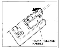
You can also open the trunk by pulling the trunk release handle to the left of the driver's seat.
