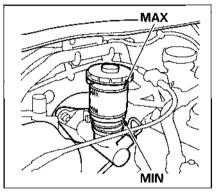
The fluid should be between the MIN and MAX marks on the side of the reservoir. If the level is at or below the MIN mark, it is an indication that your brake system needs attention. Have the brake system inspected for leaks or worn brake pads.
