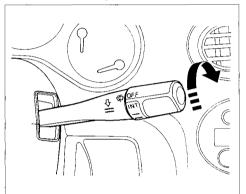
The right lever controls the windshield wipers and washers. The rotary switch at the end of the lever has three positions:
