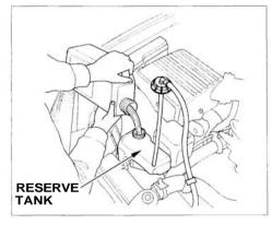
12.Fill the reserve tank to the MAX mark. Install the reserve tank cap.
