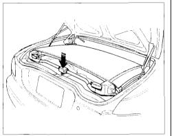
To secure the roof holder, push down on it until it locks. Make sure it is locked so it will not rattle or damage the trunk lid.
