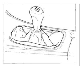
The manual transmission is synchronized in all forward gears for smooth operation. It has a lockout so you cannot shift directly from Fifth to Reverse. When shifting up or down, make sure you pusTh the clutch pedal down all the way, shift to the next gear, and let the pedal up gradually. When you are not shifting, do not rest your foot on the clutch pedal. This can cause your clutch to wear out faster.
