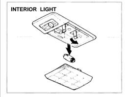
Remove the lens by carefully prying on the edge of the lens in the middle with a fingernail file or a small flat-tip screwdriver. Do not pry on the edge of the housing around the lens.
