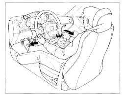
Park (P) — This position mechanically locks the transmission. Use Park whenever you are turning off or starting the engine. To shift out of Park, you must press on the brake pedal and have your foot off the accelerator pedal. Press the release button on the side of the shift lever to move it.
