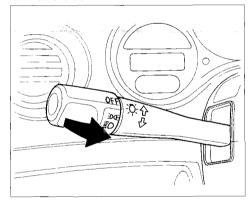
To change between low beams and high beams, pull back on the turn signal lever until you hear a click, then let go. The blue high beam indicator will light (see page 34).
