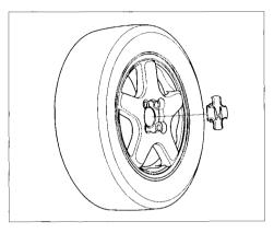
15. On the Si and VTEC models Remove the center cap before storing the flat tire in the trunk well.
