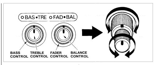
You can use the Balance control knob to turn off the illumination of the audio system. Push the Balance/ Fader controls so they pop out, then pull the Balance control knob out slightly farther.
