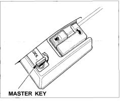
To protect items in the trunk when you need to give the key to someone else, lock the trunk release handle with the master key and give the other person the valet key.
