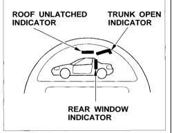
The roof and trunk monitor includes three indicators, the Roof Unlatched Indicator, the Trunk Open Indicator and the Rear Window Indicator.
