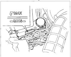
The fluid should be between the MIN and MAX marks on the side of the reservoir. If it is at or below the MIN mark, it may indicate a problem in the braking system. Have the dealer inspect your car.
