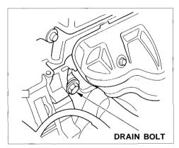
4. DOHC VTEC model only Remove the drain bolt from the engine block.
