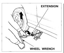
9. Use the extension and wheel wrench as shown to raise the car until the flat tire is off the ground.
