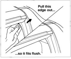
7. Check the fit of the seals at the back of the roof. If the end of either roof seal is sitting on top of the body seal, reposition the body seal.
