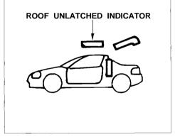
This indicator lights when you turn the ignition ON (II) if the roof panel is not fastened securely. Check both release levers to make sure they are locked.
