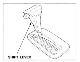
The shift lever has seven positions. It must be in Park or Neutral to start the engine. When you are stopped in D4, D3, 2, 1, N or R, press firmly on the brake pedal and keep your foot off the accelerator pedal.
