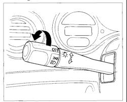
The rotating switch on the left lever controls the lights. Turning this switch to the first position " Turning this switch to the first position turns on the parking lights, taillights, instrument panel lights, side-marker lights, and rear license plate lights. Turning the switch to the second position turns on the headlights.
