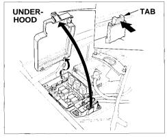
The under-hood fuse box is located in the engine compartment next to the battery. To open it, push the tab as shown.
