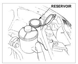
The windshield washer reservoir is located behind the left headlight. Check the reservoir's fluid level by removing the cap and looking inside.
