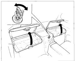
To open either rear locking compartment, put the master key in the lock, turn it counterclockwise and lift the lid up.
