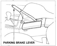
To apply the parking brake, pull the lever up fully. To release it, pull up slightly, push the button, and lower the lever. The parking brake light on the instrument panel should go out when the parking brake is fully released (see page 32). If you try to drive the car without releasing the parking brake, the ABS cannot work properly.
