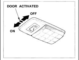
The interior light has a three-position switch. In the OFF position, the light does not come on. In the center position, the interior light comes on when you open either door. In the ON position, the interior light stays on continuously.
