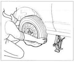
10.Remove the wheel nuts and flat tire. Temporarily place the flat tire on the ground with the outside surface of the wheel facing up. You could scratch the wheel if you put it face down.
