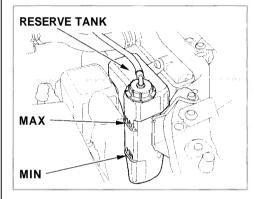
Look at the coolant level in the radiator reserve tank. Make sure it is between the MAX and MIN lines. If it is below the MIN line, see **Adding Engine Coolant** on page 131 for information on adding the proper coolant.
