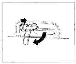
Lift the roof out of the holder. Make sure the roof panel release levers are in the unlocked (down) position.
