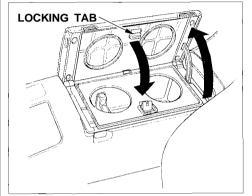
The beverage holder is located inside the center console compartment lid. To use the beverage holder, open the center console compartment. Pull the beverage holder out while pushing the locking tab.
