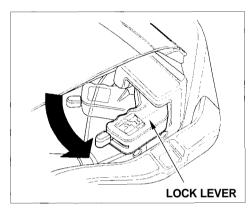
6. Lock the roof in the holder by pivoting the lock levers toward the back of the car.
