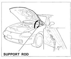
3. Pull the support rod out of its clip and insert the end into the hole on the driver's side of the hood.
