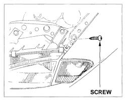
Use a Phillips-head screwdriver to remove the screw from the top of the fender.
