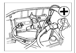
Connect one jumper cable to the positive (+) terminal on the booster battery. Connect the other end to the positive (+) terminal on your Honda's battery.
